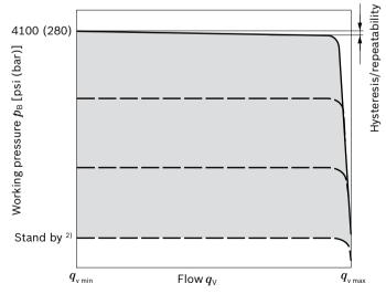
Characteristic curve valid at n<sub>1</sub> = 1500 rpm and  $\theta_{\text{fluid}}$  = 122 °F (50 °C).
