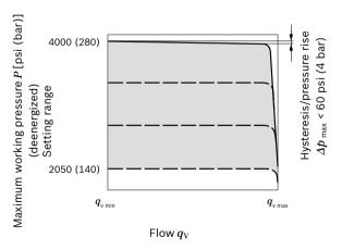
Characteristic curve valid at  $n_1$  = 1500 rpm and  $\theta_{fluid}$  = 122 °F (50 °C).
