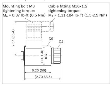
The seal ring in the cable fitting is suitable for lines of diameter 0.18 in to 0.39 in (4.5 mm to 10 mm). The mating connector is not included in the scope of delivery. This can be supplied by Bosch Rexroth on request.
