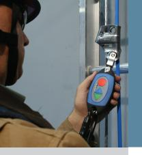
IBEX's patented continuous closed feedback loop employs a lightweight EasyClimb Controller. This simple wireless control connects the climber's body harness to the assist rope. The EasyClimb Controller transmits signals to the motor to maintain the desired level of assistance and to respond instantaneously to changes in climbing speed or direction. The field-tested controller's wireless signal seamlessly communicates climber behavior to adapt motor output for a consistent, reliable assist.
