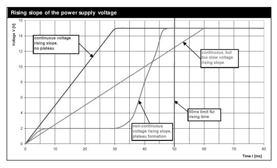
If the power supply is able to provide a higher current, a peak current will flow in the first instant to charge up the input capacitances on the driver. Its peak current value will be limited by the power supply and the effective impedances (e.g. distribution lines), only.
