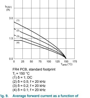
Fig. 9. ambient temperature; typical values
