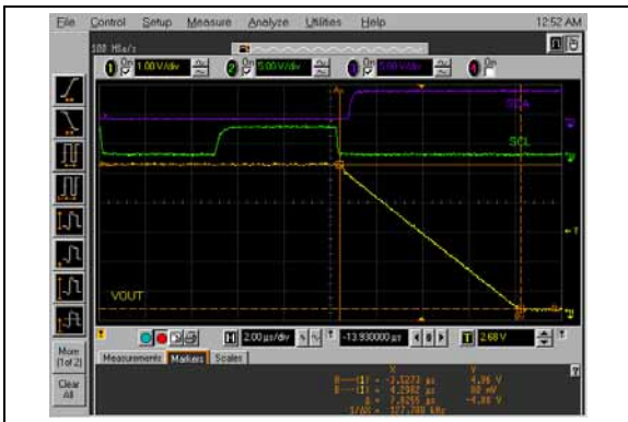
FIGURE 2-97: Full-Scale Settling Time (FFFh to 000h) (MCP4726).
