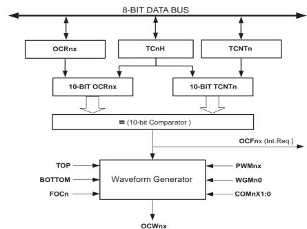
Figure 15-4. Output Compare Unit, Block Diagram
