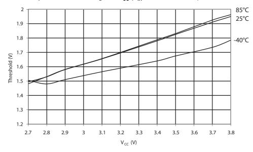
Figure 30-25. USB Pin Input Threshold Voltage vs.  $V_{CC}$  ( $V_{IL}$ , I/O Pin read as '0')
