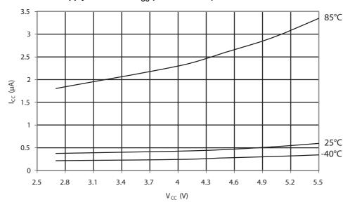
Figure 30-11. Power-Down Supply Current vs.  $V_{CC}$  (WDT Enabled)
