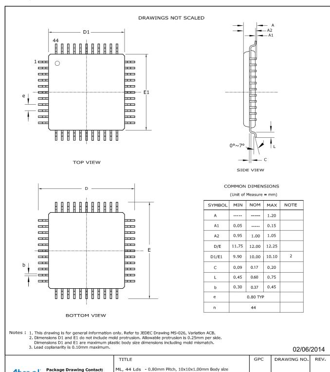
Thin Profile Plastic Quad Flat Package (TQFP)
