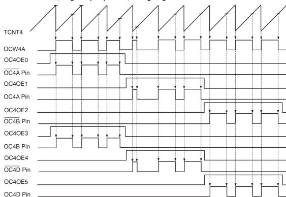
Figure 15-15. PWM6 Mode, Single-slope Operation, Timing Diagram
