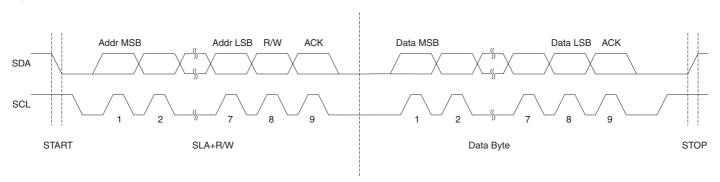
Figure 20-6. Typical Data Transmission
