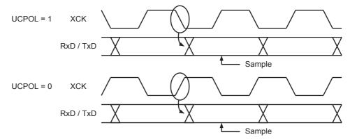
The UCPOLn bit UCRSC selects which XCKn clock edge is used for data sampling and which is used for data change. As the above figure shows, when UCPOLn is zero the data will be changed at rising XCKn edge and sampled at falling XCKn edge. If UCPOLn is set, the data will be changed at falling XCKn edge and sampled at rising XCKn edge.
