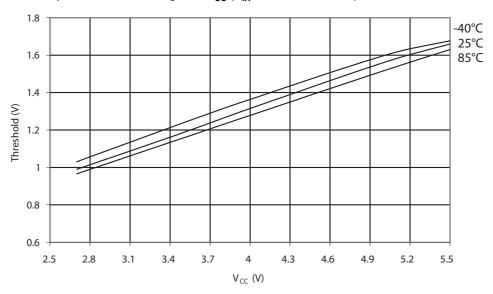
Figure 30-23. I/O Pin Input Threshold Voltage vs.  $V_{CC}$  ( $V_{IL}$ , IO Pin read as '0')
