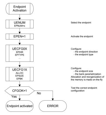
As long as the endpoint is not correctly configured (CFGOK cleared), the hardware does not acknowledge the packets sent by the host.
