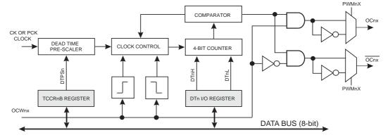
The length of the counting period is user adjustable by selecting the dead time prescaler setting by using the DTPS41:40 control bits, and selecting then the dead time value in I/O register DT4. The DT4 register consists of two 4-bit fields, DT4H and DT4L that control the dead time periods of the PWM output and its' complementary output separately in terms of the number of prescaled dead time generator clock cycles. Thus the rising edge of
