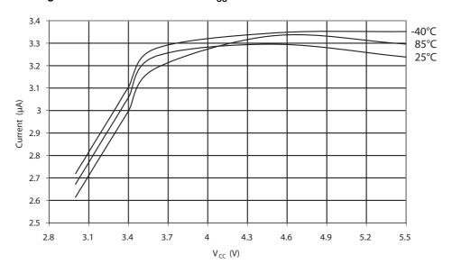
Figure 30-41. ADC Internal  $V_{REF}$  vs.  $V_{CC}$
