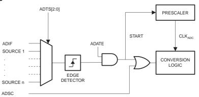
Using the ADC Interrupt Flag as a trigger source makes the ADC start a new conversion as soon as the ongoing conversion has finished. The ADC then operates in Free Running mode, constantly sampling and updating the ADC Data Register. The first conversion must be started by writing a logical one to the ADSC bit in ADCSRA. In this mode the ADC will perform successive conversions independently of whether the ADC Interrupt Flag, ADIF is cleared or not.
