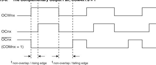
Figure 15-8. The Complementary Output Pair, COM4x1:0 = 1
