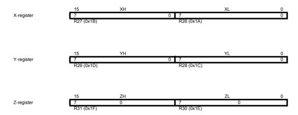
In the different addressing modes these address registers have functions as fixed displacement, automatic increment, and automatic decrement (See "Instruction Set Summary" on page 418 for detailed information).
