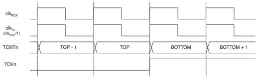
Figure 15-17. Timer/Counter Timing Diagram, with Prescaler (f<sub>clkT4</sub>/8)
