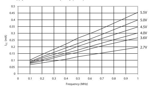
Figure 30-7. Idle Supply Current vs. Low Frequency (1MHz) and T = 85°C
