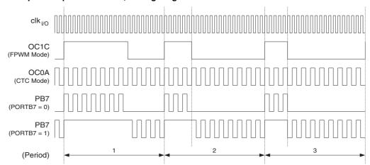
Figure 16-3. Output Compare Modulator, Timing Diagram
