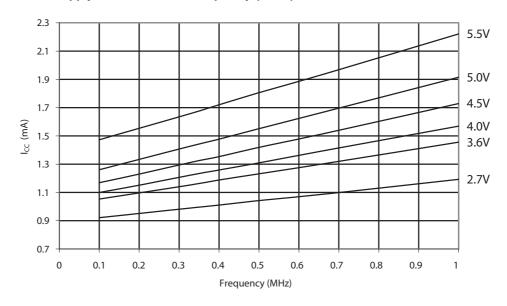
Figure 30-3. Active Supply Current vs. Frequency (1 - 16MHz) and T= -40°C
