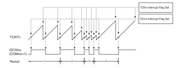
The Timer/Counter Overflow Flag (TOV4) is set in the same clock cycle as the TCNT4 becomes zero. The TOV4 Flag in this case behaves like a 11th bit, except that it is only set, not cleared. However, combined with the timer overflow interrupt, that automatically clears the TOV4 Flag, the timer resolution can be increased by software. There are no special cases to consider in the Normal mode, a new counter value can be written anytime.
