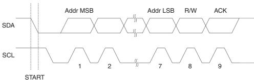
Figure 20-4. Address Packet Format
