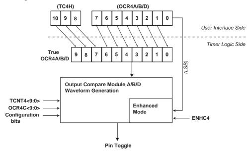
Figure 15-10 shows that the true OCR4A/B/D value corresponds to the value loaded by the user shifted on the right in order to transfer the least significant bit directly to the Waveform generation module.
