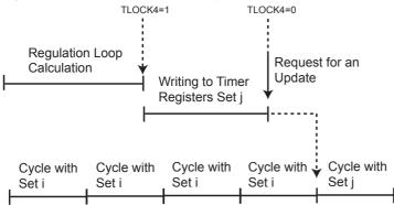
In normal operation, each write to a Compare register is effective at the end of the current cycle. But some cases require that two or more Compare registers are updated synchronously, and that may not be always possible, mostly at high speed PWM frequencies. That may result in some PWM periods with incoherent values.
