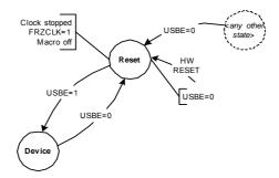
USB Controller state after an hardware reset is 'Reset'. In this state:
