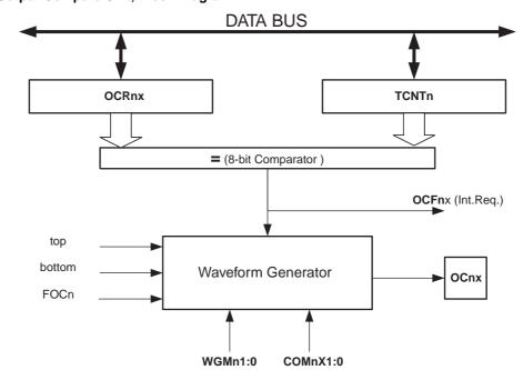
Figure 13-3. Output Compare Unit, Block Diagram
