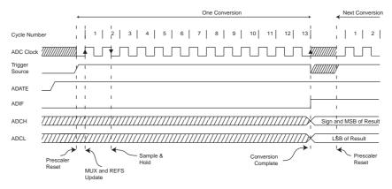
Figure 24-7. ADC Timing Diagram, Free Running Conversion
