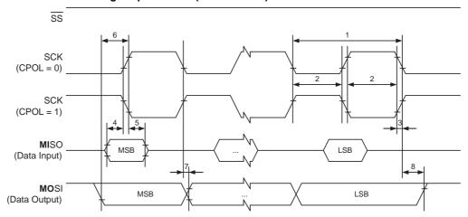
Figure 29-5. SPI Interface Timing Requirements (Slave Mode)
