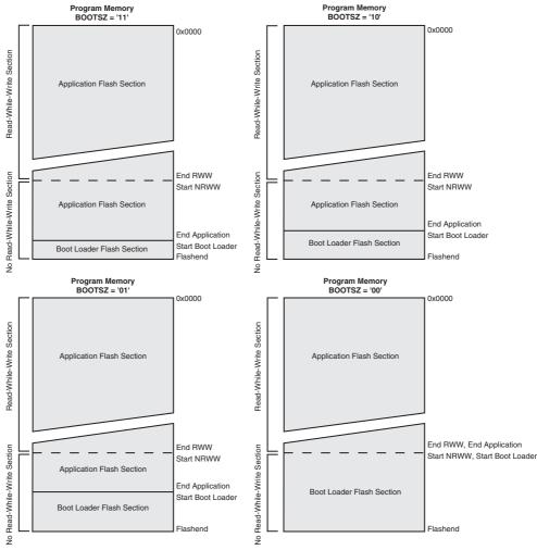
Note: 1. The parameters in Figure 27-2 are given in Table 27-8 on page 349.
