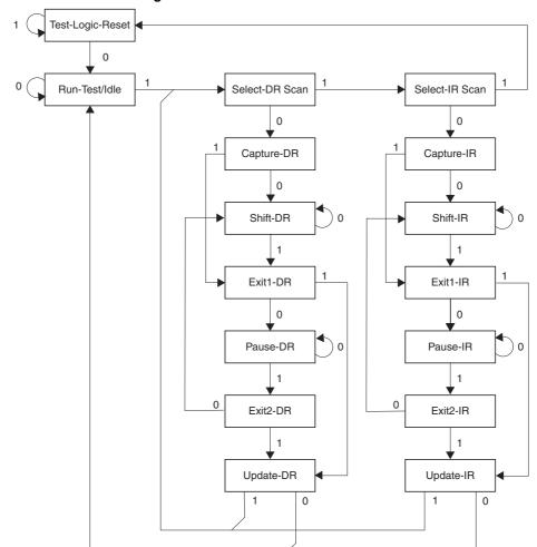
Figure 25-2. TAP Controller State Diagram
