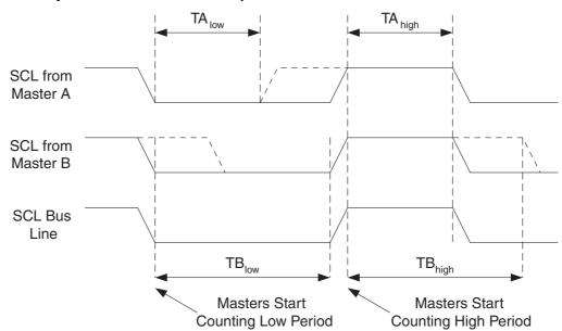
Figure 20-7. SCL Synchronization Between Multiple Masters
