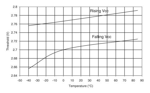
Figure 30-29. BOD Thresholds vs. Temperature (BODLEVEL is 3.5V)
