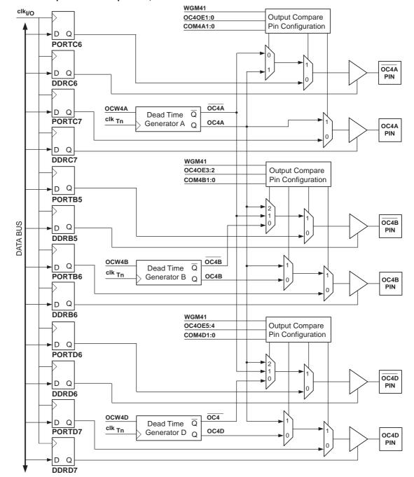
Figure 15-9. Compare Match Output Unit, Schematic
