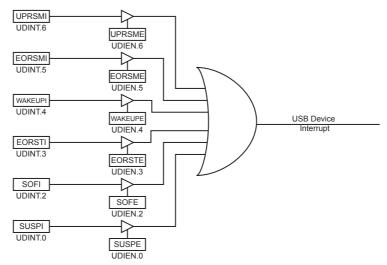
There are two kind of interrupts: processing (i.e. their generation are part of the normal processing) and exception (errors).
