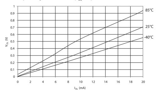
Figure 30-19. I/O Pin Output Voltage vs. Source Current ( $V_{CC} = 3V$ )
