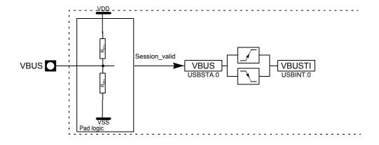
The control logic of the VBUS pad outputs a signal regarding the VBUS voltage level:
