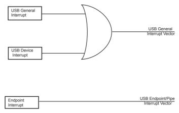
The USB hardware module distinguishes between USB General events and USB Endpoint events that are relevant with data transfers relative to each endpoint.
