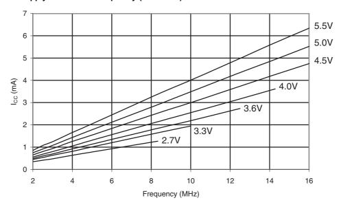
Figure 30-9. Idle Supply Current vs. Frequency (1 - 16MHz) T = 85°C
