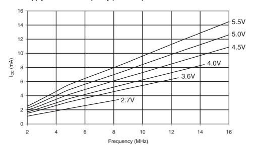
Figure 30-5. Active Supply Current vs. Frequency (1 - 16MHz) and T = 85°C
