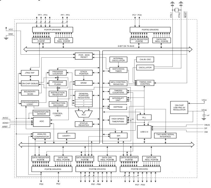
The AVR core combines a rich instruction set with 32 general purpose working registers. All the 32 registers are directly connected to the Arithmetic Logic Unit (ALU), allowing two independent registers to be accessed in one single instruction executed in one clock cycle. The resulting architecture is more code efficient while achieving throughputs up to ten times faster than conventional CISC microcontrollers.
