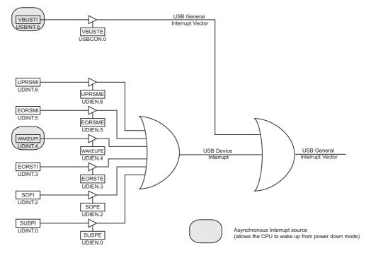
Almost all these interrupts are time-relative events that will be detected only if the USB clock is enabled (FRZCLK bit set), except for:
