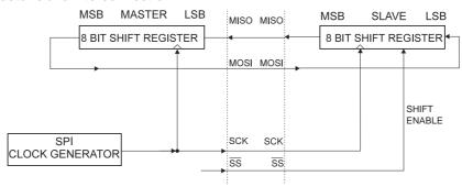
The system is single buffered in the transmit direction and double buffered in the receive direction. This means that bytes to be transmitted cannot be written to the SPI Data Register before the entire shift cycle is completed. When receiving data, however, a received character must be read from the SPI Data Register before the next character has been completely shifted in. Otherwise, the first byte is lost.
